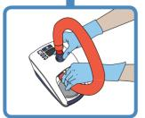
Connect the red end of the disinfection tube to the left-hand chamber port as shown and push fully into position.
