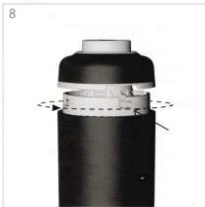
To reassemble, ensure that the O-ring is seated in the groove at the bottom of the end cap, align the pins on the end-cap, and push downwards, and twist slightly counter-clockwise until the pins return to the locked position. Finally, replace the retaining clip by firmly pressing straight down until it "clicks" into place.
