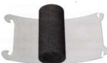
Take the new inner foam baffle material and place this on top of the plastic sleeve liner. Roll the foam material so that the edges of the plastic sleeve liner meet and the tabs are adjacent to each other. Once the tabs are aligned, slip one of the tabs past the other such that they interlock.
