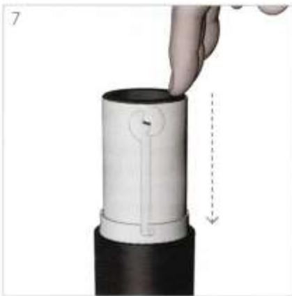
Insert the rolled inner foam baffling material into the body of the Qtube and push all the way until the bottom of the material contacts the opposite end of the Qtube body. You should be able to look down the center of the material and see that the center is clear and that there are no obstructions to the airflow.
